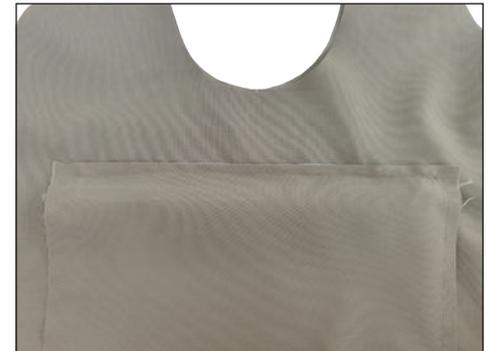
Turn the piece over and sew the „Pocket bag“ inside pocket lining to the zipper from the front. To do this, sew the top long seam again along the zipper. Note: The inside pocket lining must be placed so that only one seam allowance is sewn on and not the inside pocket.
